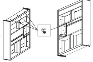
6. Remove the screw on electricall box of the cabinet
