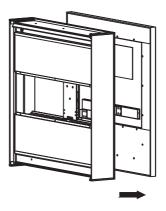
$6\,$  .Remove the screw connecting the door to the back plate on the door,take out the back plate .
